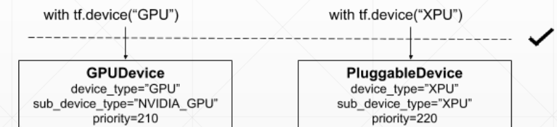
Scenario 2: Single PluggableDevice registered as a new device type, e.g., "XPU"
